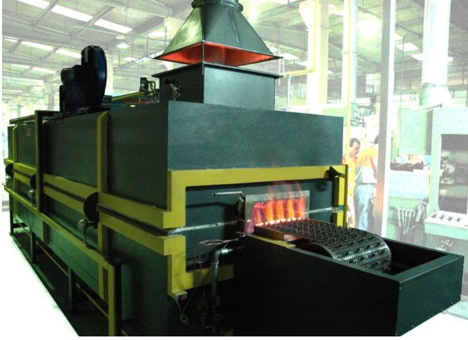
TEL BANT KONVEYÖRLÜ ATMOSFER KONTROLLÜ TAV FIRINI MESH BELT ANNEALING FURNACE WITH CONTROLLED ATMOSPHERE
